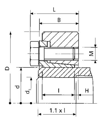
B mm = 18.0 d H8 mm = 26 D mm = 51.5 ds mm = 20 F kN torque = 23 H = 2.0 I mm = 15.0 L mm = 22.0  $\begin{array}{ll} \text{M mm} & = \text{M6} \\ \text{T N m torque} & = 230 \\ \text{Ts N m bolt tightening torque} = 13 \\ \end{array}$
